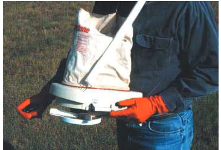
Figure 3. Hand-held bag spreader for fire ant treatment application. Credits: C. Barr
